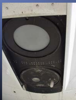
2 coverable large openings in the bottom of fuselage (515 mm diameter)
