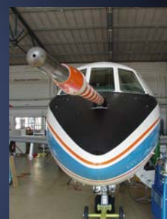
nose boom with flow angle sensor (CFK, 1.8 m length)
