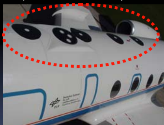
1 large opening on top of fuselage (515 mm diameter), (added in 1997)
