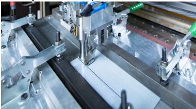
Flat specimen welding (PPS, PEEK, PEKK)
