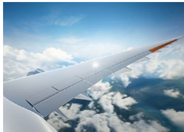
06 High-aspect-ratio wing with multi-functional control surfaces
