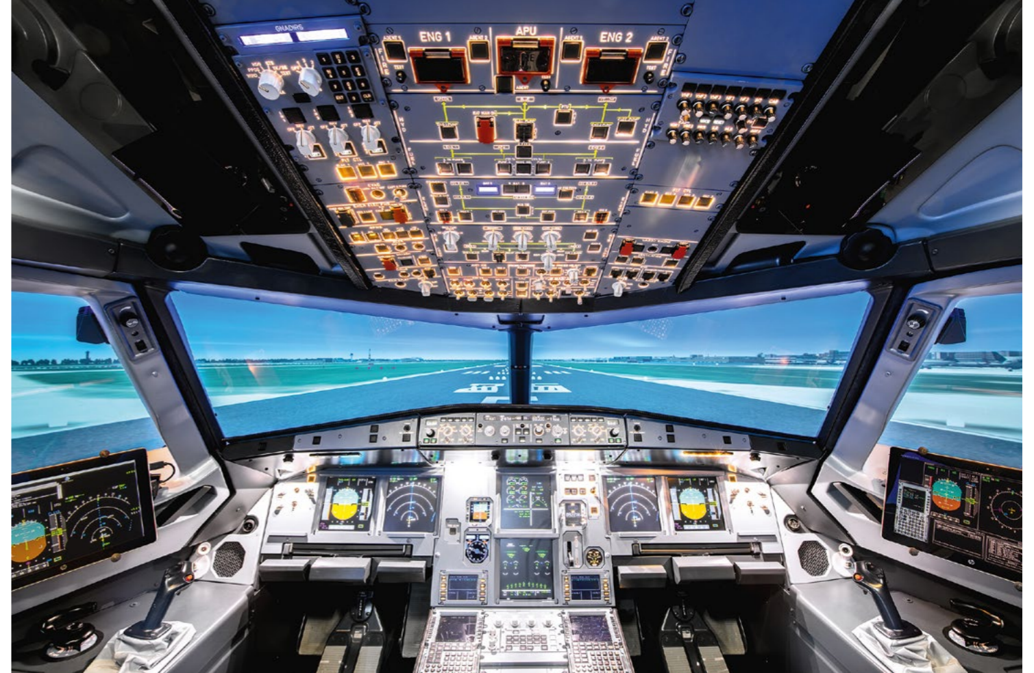
A320 cockpit module with additional displays, including those for the LNAS pilot assistance system.
